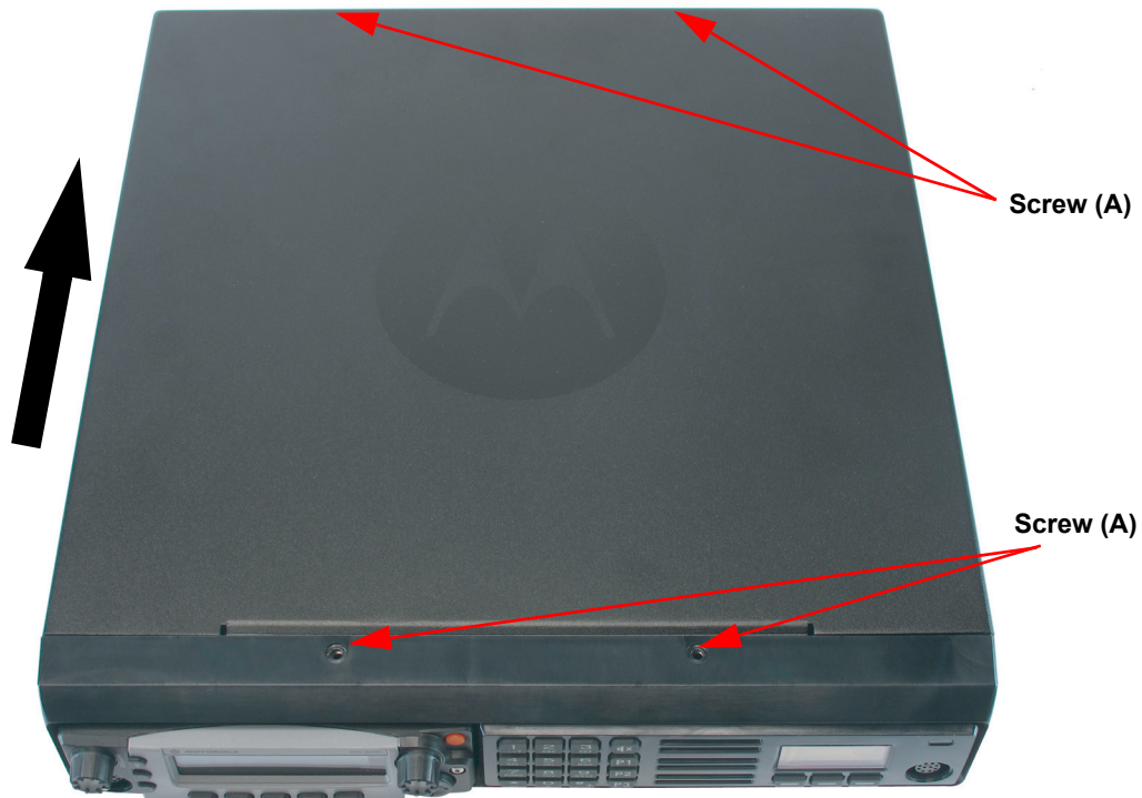
Figure 5-1. Removing and Replacing the Top Cover
